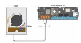
The Alarm Panel Pro has two dedicated 12V siren outputs. Connect the red wire to 12V+ and black wire to ALRM1- or ALRM2-
