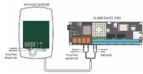
Motion sensors have 4 wires: A red and black wire for 12V power is connected to AUX+ and AUX-
